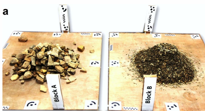
Fig. 22. Experimental setups of (a) two initial ice-cemented blocks, and (b) a frozen block degrading in the water tank.
