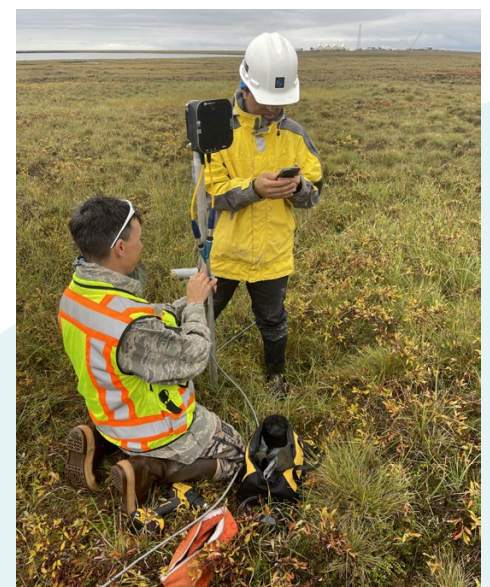
Beadedstream's D605 remote data loggers being installed for ice road monitoring.
