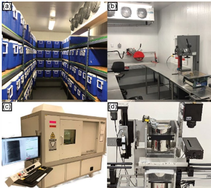
PACS Lab equipment: (a) archive freezer, (b) cutting/core processing room, (c) Nikon XTH 225 Industrial CT Scanner, and (d) Geotek multi-sensor core logger.
