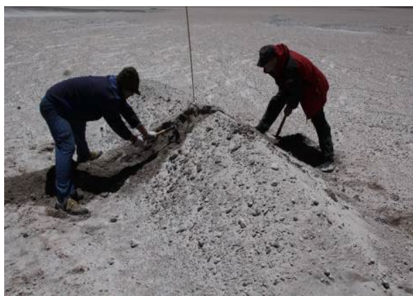
Figure 6. Physical sounding of permafrost table (see metal avalanche probe sticking in sediment) and clearing of cryoforms from sedimentary veneer.
