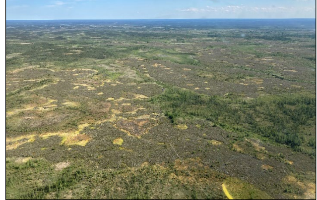
Figure 13. Widespread permafrost thaw (thermokarst) along the Nelson River in Manitoba.
