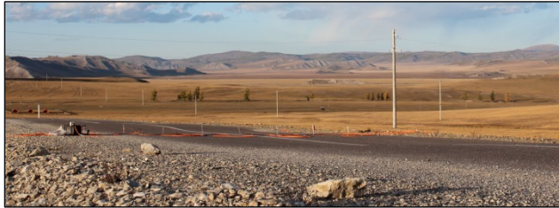
Figure 3. ERT survey across the road, Wenner-Schlumberger array with 1 m spacing
