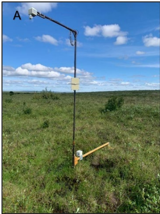
Figure 2. (A) Ultrasonic snow depth sensor and (B) inclinometer. The center pole is mounted into the permafrost such that it remains stationary.
