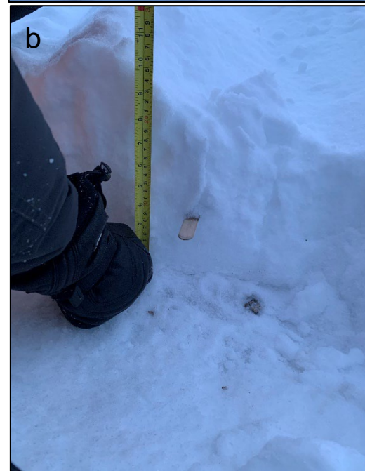
Figure 4. Snow pits dug at the M2 (a) undisturbed plot, with a depth of 53 cm and (b) compacted plot, with a depth of 23 cm, on 5 January 2021, after the second compaction.
