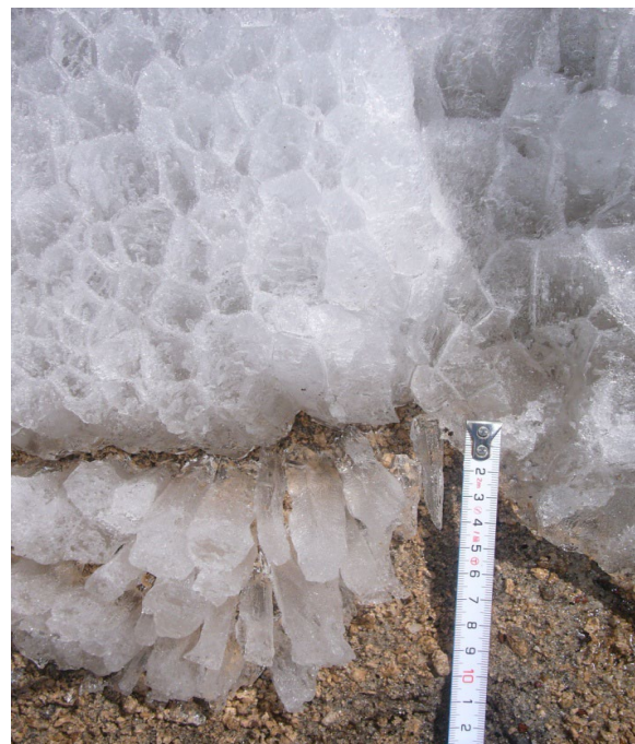
Figure 12. Typical hexagonal ice crystals in the top layer of the permafrost showing sizes up to 12 cm length and 3 cm in diameter.
