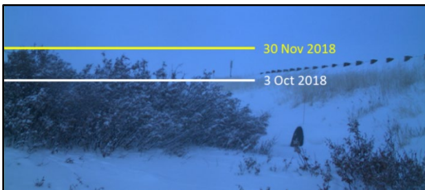
Figure 2. Riparian terrain upstream of a culvert near Tuktoyaktuk, 30 Nov 2018. The lines indicate the tops of the willows on 3 Oct and 30 Nov. Total heave over this period was approximately 1 metre.
