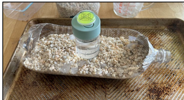
Figure 3. Setup of the hands-on activity in “Observing Impacts to Communities Built on Permafrost.” Students pour hot water (simulating a warming climate) and observe changes to a model house sitting on ice and gravel (simulating soil containing permafrost).
