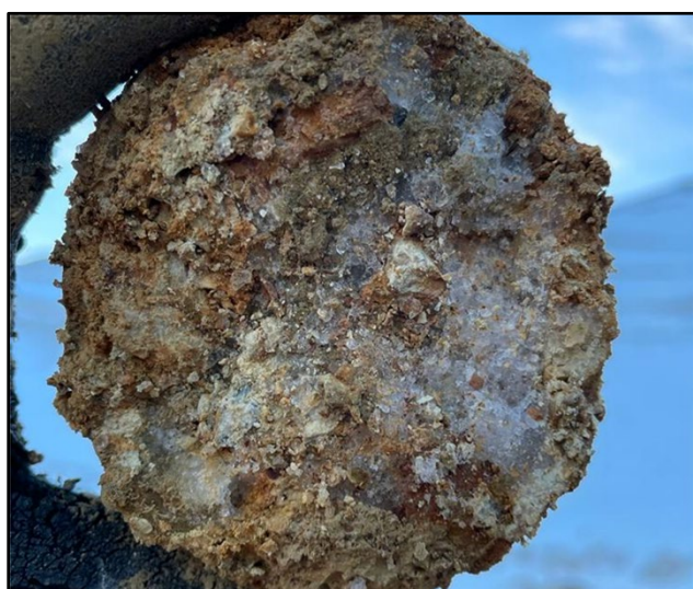
Photography 1. GE_01 sonic drilling sample (ground ice).
