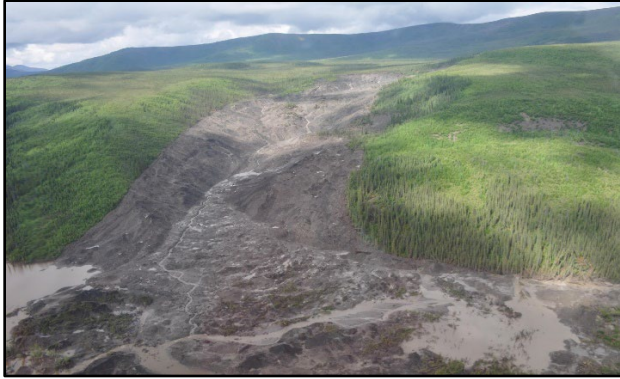
Figure 1. Oblique view of the Redstone River PDS. The width of the scar zone is approximately 375 m.
