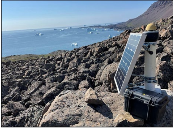
Figure 2. Surface of Apostelfjeld rockglacier with fixed GNSS station in the foreground. Results
