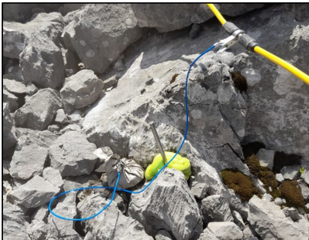
Figure 1. Example of a stainless-steel electrode hammered in between the boulders, coupled with salt water-soaked sponges, and a conductive textile sachet electrode placed between the boulders and moistened with salt water (image taken at the Marocche di Drò test site).
