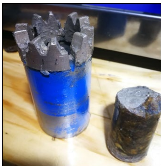
Figure 2. Recovered piece of the frozen subglacial bedrock core and impregnated diamond drill bit used for coring (from Talalay et al. 2021b).
