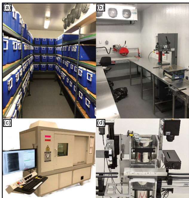
Figure 1. (a) image of PACS Lab archive freezer, (b) image of PACS Lab cutting/core processing room, (c) Nikon XTH 225 ST Industrial CT Scanner (d) Geotek MSCL.
